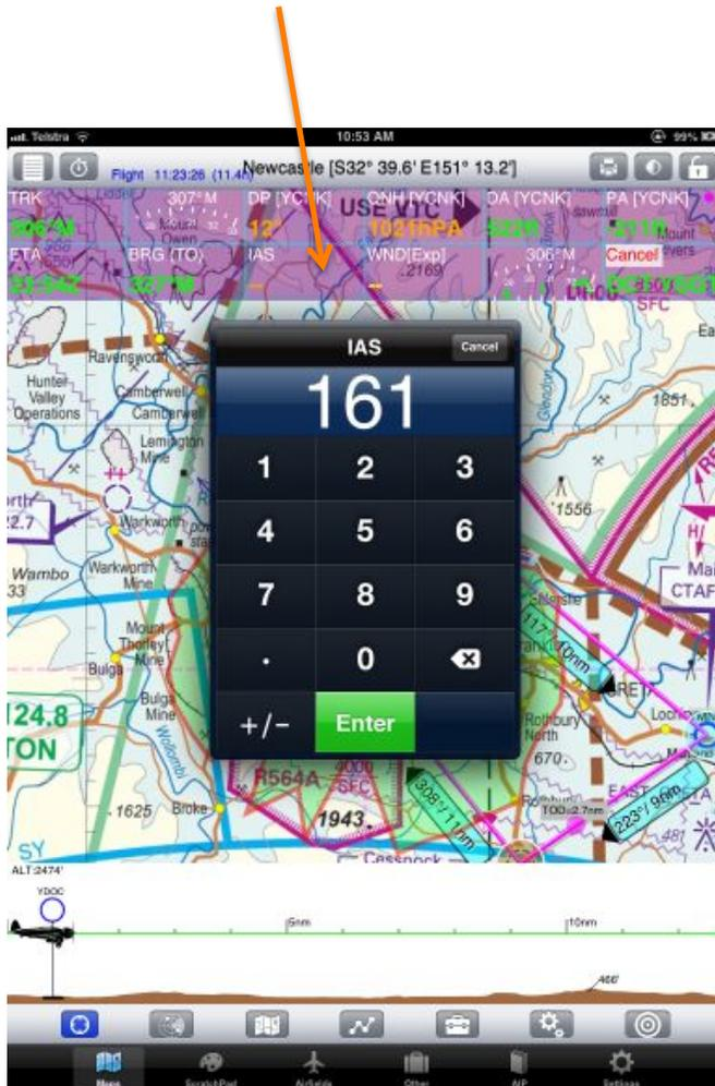
We have included an experimental wind calculator. It requires you to set the IAS at any particular time you need an estimate of the wind. We have found that the wind speed is generally within 5kts and the direction within 20 degrees. The value is highlighted in yellow to indicate it is very experimental. If it proves useful we will leave it in.
